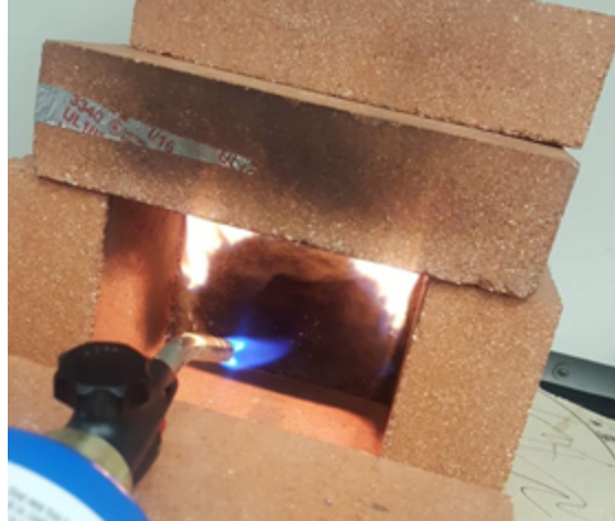
Figure 13: Lab Created Forge for Thermal Testing
